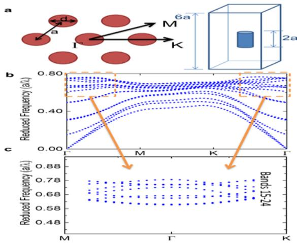
**FIGURE 2.** Modeling of the photonic band structure of the photonic crystal lasers.
