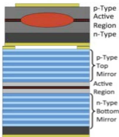
**FIGURE 1.** (Top) Conventional edge-emitter viewed from facet; and (Bottom) Conventional VCSEL viewed from side. Figure courtesy Siriani D., the new look of semiconductor lasers, CLEO Conference, Science and Innovations, <http://blog.cleoconference.org/2013/02/the-new-look-of-semiconductor-lasers/>.
