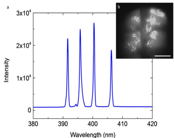
**FIGURE 4.** Four photonic crystal laser “pixels” operating together in close vicinity (The scale bar represents  $10 \mu\text{m}$ ). Figure courtesy Wright *et al.*, Multi-Colour Nanowire Photonic Crystal Laser Pixels, <http://www.nature.com/srep/2013/131018/srep02982/full/srrep02982.html>.
