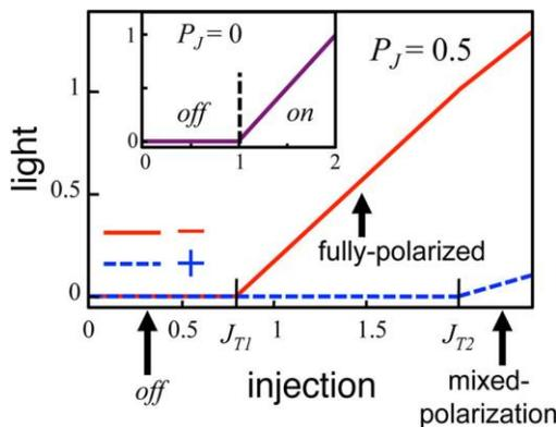
**FIGURE 3.** The variation of the emitted light intensity with the injection intensity for spin lasers ( $P_J \neq 0.5$ ) and conventional lasers ( $P_J = 0$ , inset). Figure courtesy Boeris G., Lee J., Vyborny K., and Žutić I., *Tailoring chirp in spin-lasers*, Appl. Phys. Lett. **100**, 121111 (2012).
