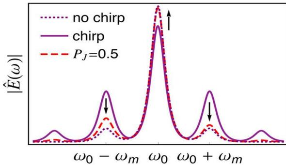
**FIGURE 5.** Broadened spectra of electric fields  $|\hat{E}(\omega)|$ , of a laser with optical frequency  $\omega_0$  where  $\omega_m$  is modulation frequency. The conventional lasers with chirp and without chirp and a spin laser with spin injection are shown respectively by dotted line, solid line, and dashed line. Figure courtesy Boéris G., Lee J., Výborný K., and Žutić I., *Tailoring chirp in spin-lasers*, Appl. Phys. Lett. **100**, 121111 (2012).
