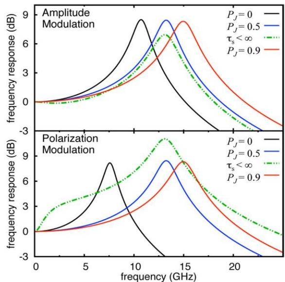
**FIGURE 4** Frequency response with different polarizations. Figure courtesy Lee J., Falls W., Oszałdowski R. and Žutić I., *Spin modulation in semiconductor lasers*, Appl. Phys. Lett. **97**, 041116 (2010).
