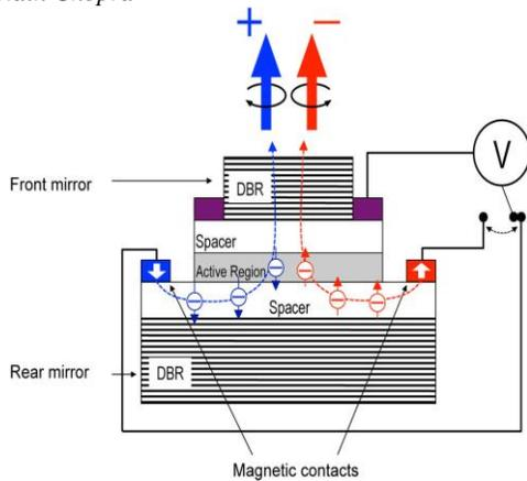
**FIGURE 2** Schematic illustration of a spin laser structure with vertical cavity surface emitting laser (VCSEL) geometry. Figure courtesy spie.org.
