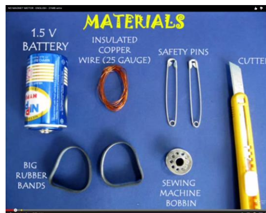
FIGURE 2. Materials needed to make a magnetic motor powered by electromagnet [11].
