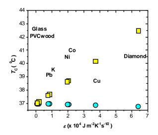
**FIGURE 2.** Contact temperatures as a function of thermal effusivity when touching with the hand at 37  $^{\circ}$ C objects of different materials at 0  $^{\circ}$ C (blue circles) and 1000 $^{\circ}$ C (yellow squares).
