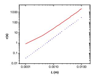
**FIGURE 3.** The time  $\tau$  required for the skin to reach values of the contact temperature of 0<sup>o</sup>C and 100<sup>o</sup>C without frostbitten or burning up respectively (see text), as a function of the hypothetical thickness of the gas layer evaporated at the surface. The solid (red) and dotted (blue) curves correspond to the case of touching a cold (-196<sup>o</sup>C) and a hot (600<sup>o</sup>C) object, respectively.
