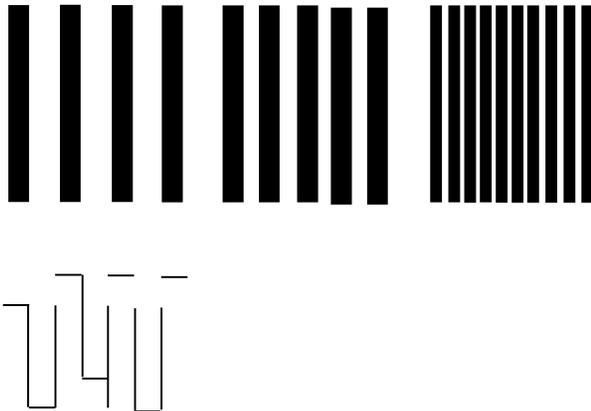
FIGURE 5. Sine wave and square wave grating.
