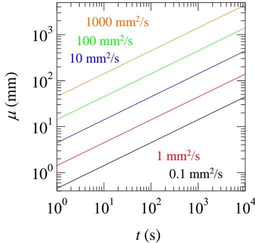
**FIGURE 3.** Penetration depth of heat as a function of time according to Eq. (17) in logarithmic scale. Five thermal diffusivities are considered.
