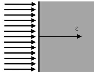
FIGURE 1. Diagram of an opaque and semi-infinite sample whose surface ( $z = 0$ ) is uniformly heated.
