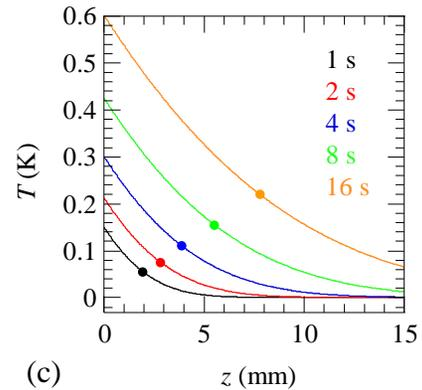
**FIGURE 2.** (a) Depth dependence of the temperature of a semi-infinite block of stainless steel whose free surface is put in contact with a thermal reservoir at 10 K. Six times are plotted. (b) The same when the steel block is illuminated by a brief flash lighting of 25 kJ/m<sup>2</sup>. (c) The same when the steel block is illuminated by a continuous light beam of intensity 1 kW/m<sup>2</sup>. Dots indicate the thermal diffusion length at each time.
