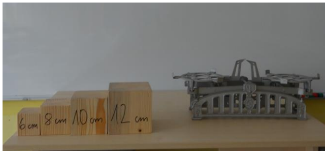
FIGURE 5. Four cubes and the balance given to students for hands-on activity to find the equilibrium configuration.
