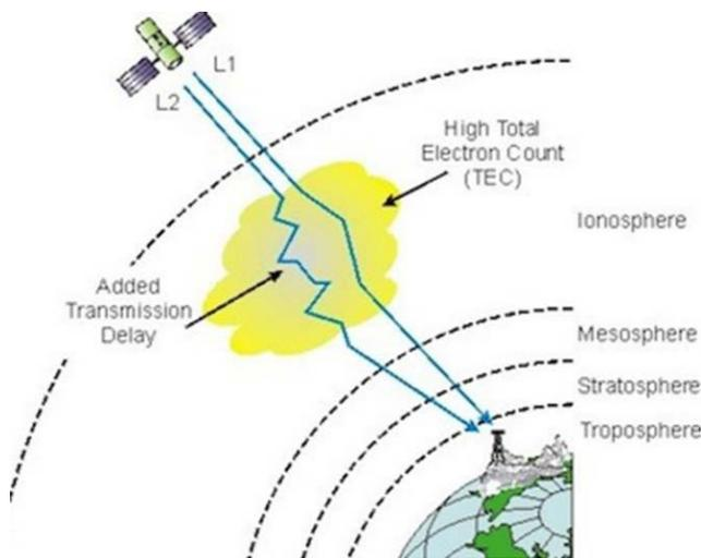
FIGURE 1.1b: Effect of the ionosphere on GPS signals (after [3]).
