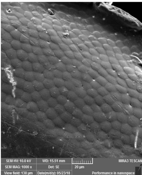
**FIGURE 4.** Microphotograph of the room temperature exoskeleton of *Phanaeus kirbyi* using scanning electron microscopy (SEM). Typical length of each polygon is about 10 $\mu$ m.
