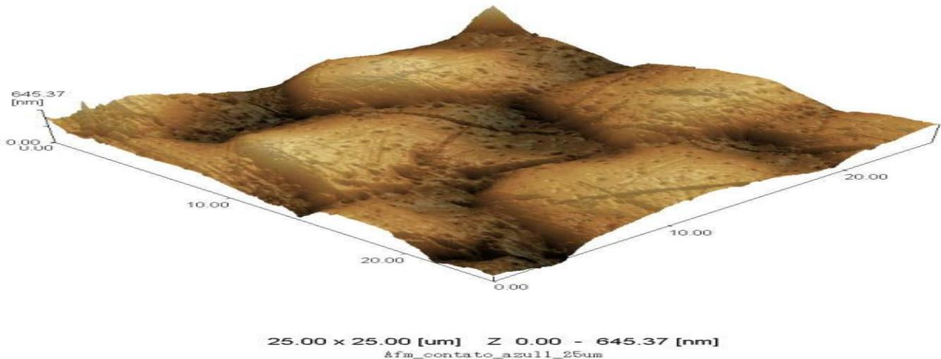
**FIGURE 3.** Image of the room temperature exoskeleton of *Phanaeus kirbyi* from contact mode of atomic force microscopy (AFM). Helical structures are not evident, at the surface.
