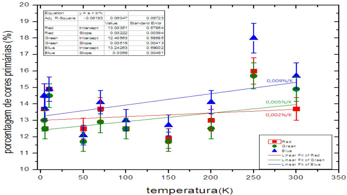
**FIGURE 2.** Variation, with temperature, of the color of the exoskeleton of *Phanaeus kirbyi*. RGB color system, with the linear adjustment of the percentages of the primary colors red, green and blue.
