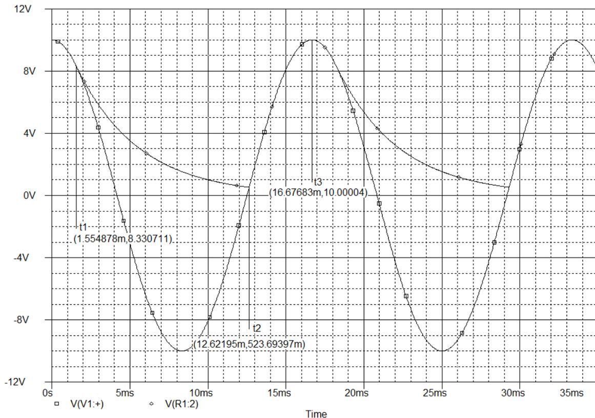
**FIGURE 3.** Simulated input ac voltage ( $V(V1:+)$ ) and voltage across the capacitor ( $V(R1:2)$ ) of Fig. 1 for the extremely high ripple case, *i.e.*,  $r = 0.95$ .
