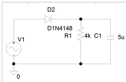
**FIGURE 1.** PSpice circuit diagram of a half-wave rectifier.
