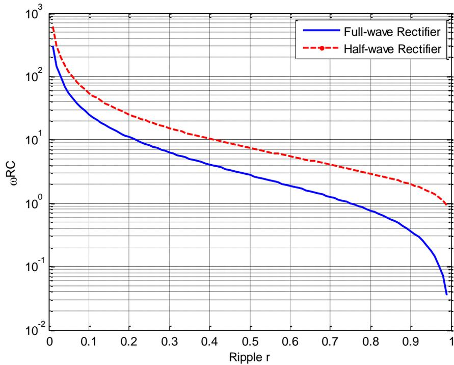
FIGURE 4. Numerical solution of Eq. (14) for the half-wave rectifier and Eq. (22) for the full-wave rectifier.
