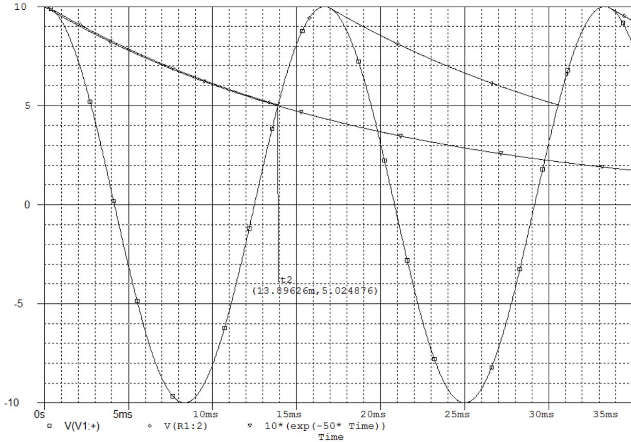
FIGURE 6. Simulated input ac voltage  $V(V1: +)$  and voltage across the capacitor  $V(R1:2)$  of Fig. 1 for high ripple case, *i.e.*,  $r = 0.5$ . Also shown is the exponential voltage  $10e^{-50t}$   $V$  which approximates the voltage across the capacitor quite well, for  $0 \leq t \leq t_2$ .
