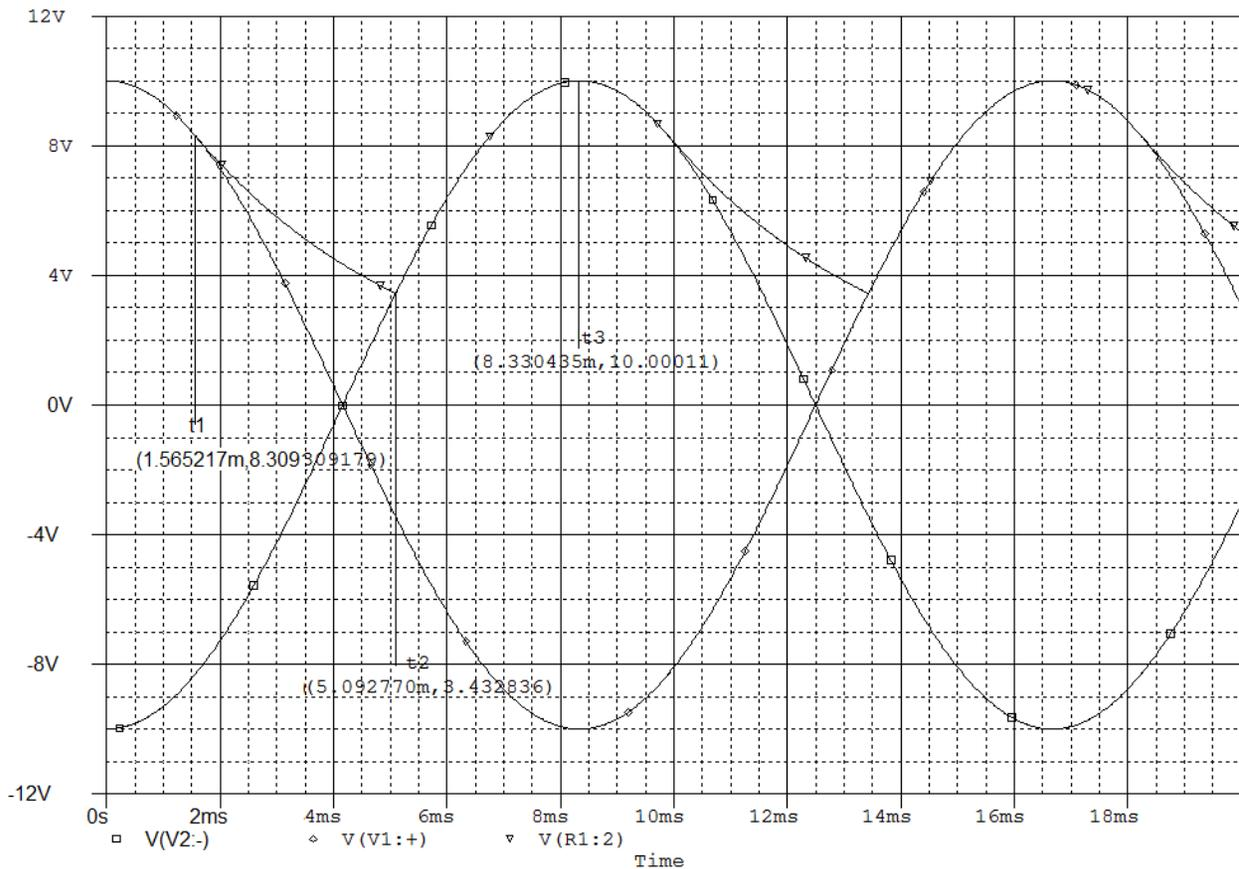
FIGURE 5. Simulated input ac voltages ( $V(V1: +)$ ) and ( $V(V2: -)$ ), and voltage across the capacitor ( $V(R1: 2)$ ) of Fig. 2, for the extremely high ripple case, i.e.,  $r = 0.66$ .
