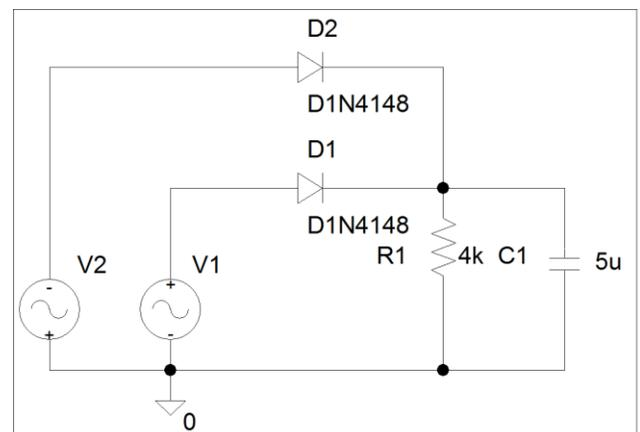
**FIGURE 2.** PSpice circuit diagram of a full-wave rectifier.
