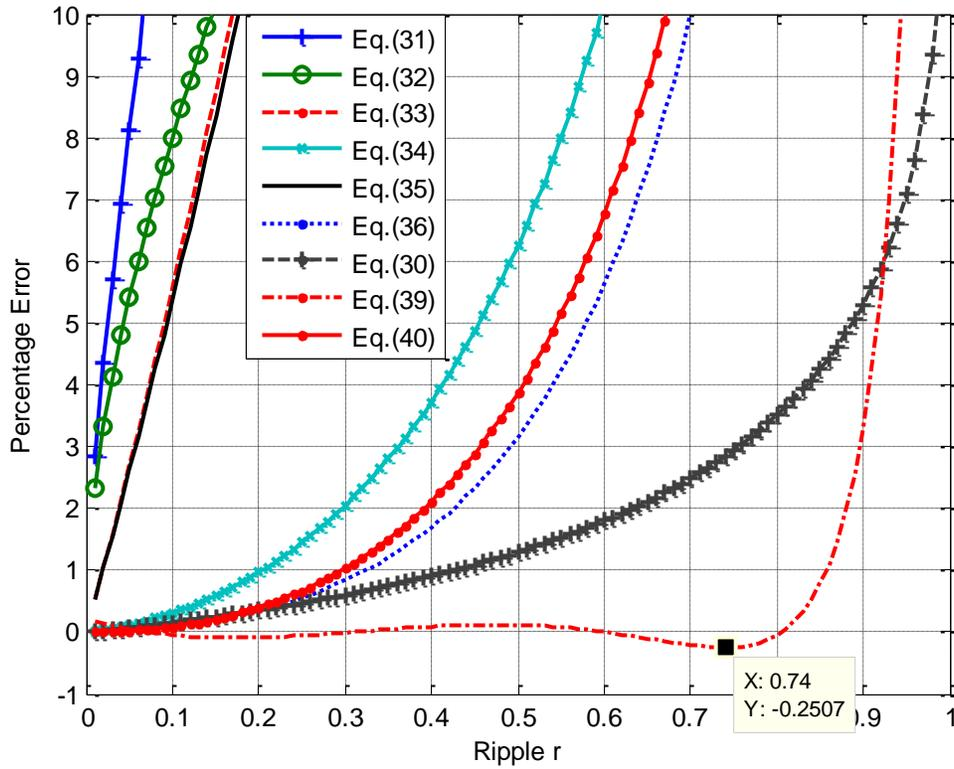
FIGURE 8. Percentage errors of Eq. (30) to Eq. (36), Eq. (39) and Eq. (40), relative to the numerical solution of Eq. (14), for the half-wave rectifier.
