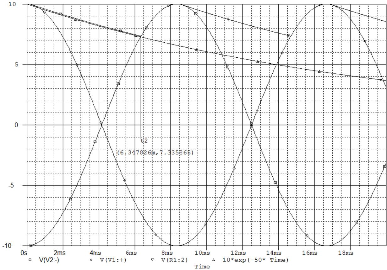
**FIGURE 7.** Simulated input ac voltages (V(V1:+)) and (V(V2:-)), and the voltage across the capacitor (V(R1:2)) of Fig. 2 for high ripple case, *i.e.*,  $r = 0.27$ . Also shown is the exponential voltage  $10e^{-50t}$  V which approximates the voltage across the capacitor quite well, for  $0 \leq t \leq t_2$ .
