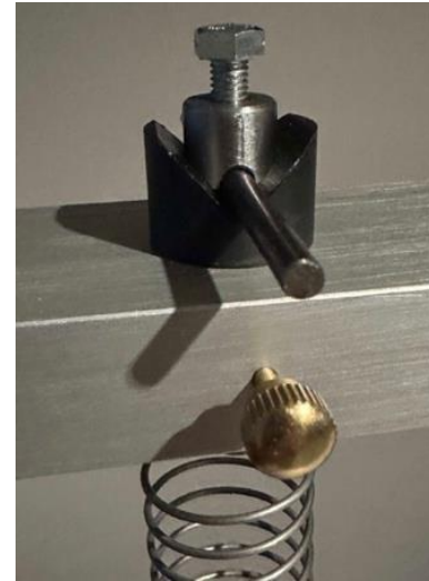
FIGURE 2. Roto-translational suspension device.
