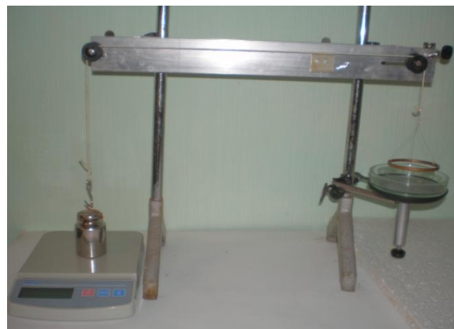
FIGURE 4. The experimental installation for determination of surface tension of liquids.
