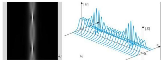
**FIGURE 8.** a) Gray tones represents the light intensity produced by two solitons propagating very closely and with the same phases through a nonlinear waveguide. b) Transversal sections of the electric field intensity for the solitons propagation in a).
