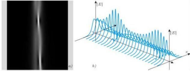
**FIGURE 9.** a) Gray tones represents the light intensity produced by two solitons propagating very closely and with a phase difference of  $\pi/4$  through a nonlinear waveguide. b) Transversal sections of the electric field intensity for the solitons propagation in a).
