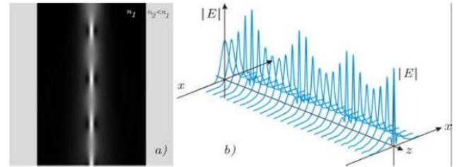
**FIGURE 3.** a) Graph in gray tones represent the laser intensity propagating through a guide with cubic parameter  $a_3 = 3000$ . b) Progressive section from the electric field intensity propagating in a self-refractive media with positive cubic parameter.
