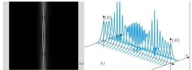
**FIGURE 7.** a) Gray tones represents the light intensity produced by a three-soliton propagating through a nonlinear waveguide. b) Transversal sections of the electric field intensity for the three-soliton propagation.
