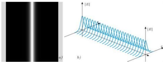
**FIGURE 5.** a) Gray tones represents the light intensity produced by a soliton propagating through a nonlinear waveguide. b) Transversal sections of the electric field intensity for the soliton propagation.
