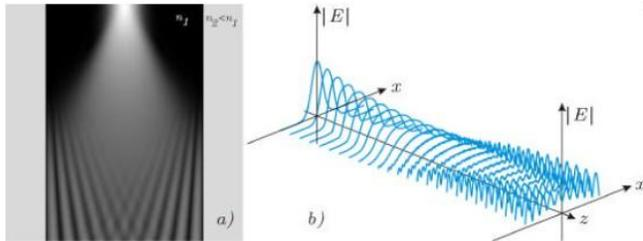
**FIGURE 2.** a) The gray tones represents the laser intensity propagating in a waveguide with cubic parameter equal to -3000.0. b) Transversal sections of the electric field intensity for the propagation in a self-refractive media with negative cubic parameter.
