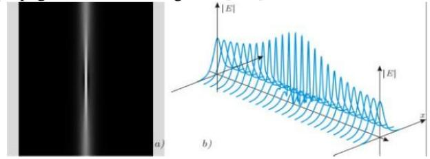
**FIGURE 6.** a) Gray tones represents the light intensity produced by a two-soliton propagating through a nonlinear waveguide. b) Transversal sections of the electric field intensity for the two-soliton propagation.
