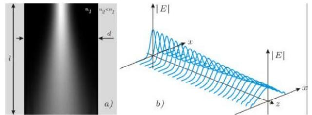
**FIGURE 1.** a) This graphic represents the laser intensity that propagate through a waveguide with constant refractive index. The plot in b) shows the transversal sections magnitude of the electric field for the propagation of light in the linear media.
