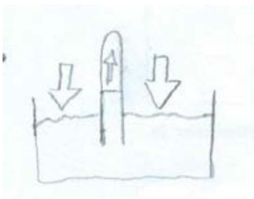
**FIGURE 9.** Another schematic presentation of the Torricelli experiment.
