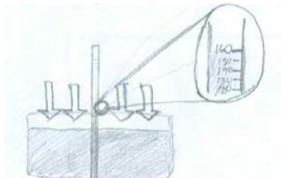
**FIGURE 10.** Another schematic presentation of Torricelli experiment with a zoom.
