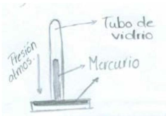
**FIGURE 8.** A schematic presentation of Torricelli experiment (Presión atmos. = atmospheric pressure; Tubo de vidrio = glass tube; Mercurio = mercury).
