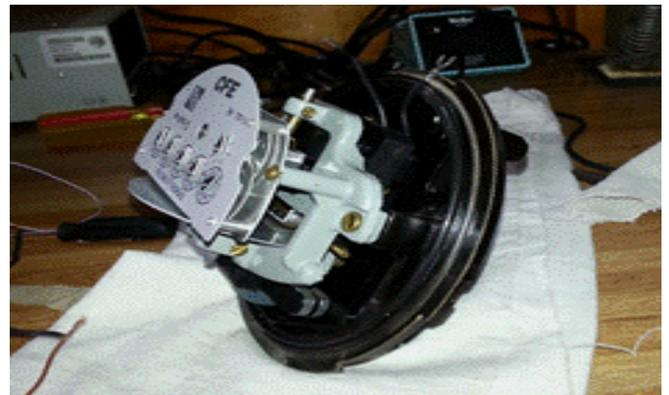
**FIGURE 6.** Traditional household electricity AC energy meter with its front cover removed.
