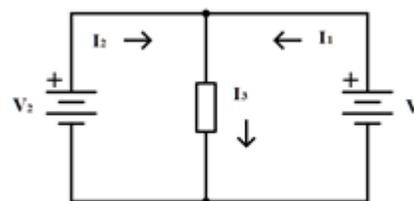
**FIGURE 1.** Two batteries in parallel sharing a load.
