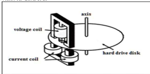
FIGURE 7. Electromagnetic induction disk meter outline.
