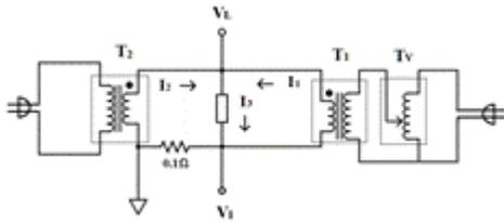
**FIGURE 4.** Inserting a low value resistor for I2 phase monitoring.
