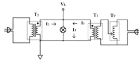
**FIGURE 3.** Two transformers in parallel powering a lamp.
