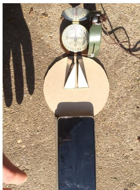
FIGURE 5. Checking the solar noon with a home-made "slotted" sundial and a compass.
