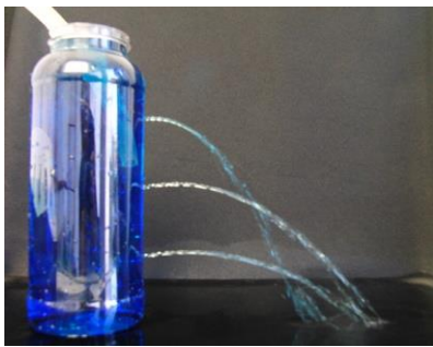
FIGURE 10. The jets when the holes' diameter is 1.984 mm (5/64 in or 5/64 in).
