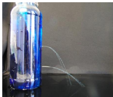
FIGURE 8. The jets when the holes' diameter is 0.794 mm (1/32 in or 2/64 in).
