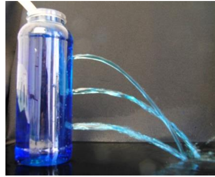
FIGURE 13. The jets when the holes' diameter is 6.35 mm (1/4 in or 16/64 in).
