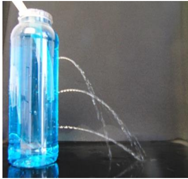
FIGURE 9. The jets when the holes' diameter is 1.587 mm (1/16 in or 4/64 in).
