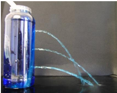
FIGURE 11. The jets when the holes' diameter 3.175 mm (1/8 in or 8/64 in).
