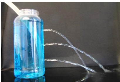
FIGURE 12. The jets when the holes' diameter is 4.762 mm (3/16 in or 12/64 in).
